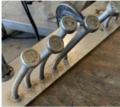
Figure 6, 3/8" studs on 7 gauge 304 base material
