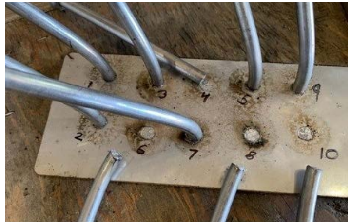
Figure 9, Next eight studs after the first two studs passed preproduction testing
