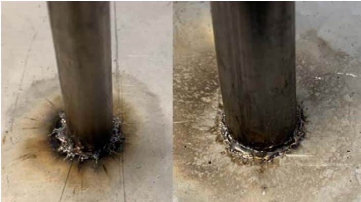
Figure 10, Left: No anti-spatter applied. Right: Water-based anti-spatter applied
