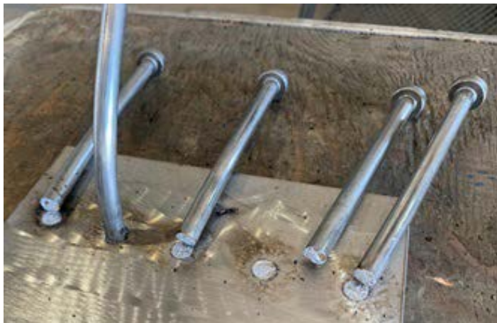
Figure 6, 3/8" studs on 7 gauge 304 base material
